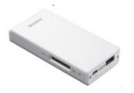
The Sony WG-C10 Portable Wireless Server http://www.sony.net/Products/ws/en\_us/pwsintro; \$80) does all the Smartbox does for eight simultaneous users, and adds a port to share a USB Flash drive.
