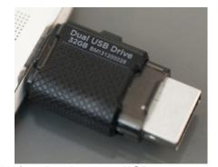
In this context, a dual USB drive is a device that has two USB connectors. In the case of the SanDisk
