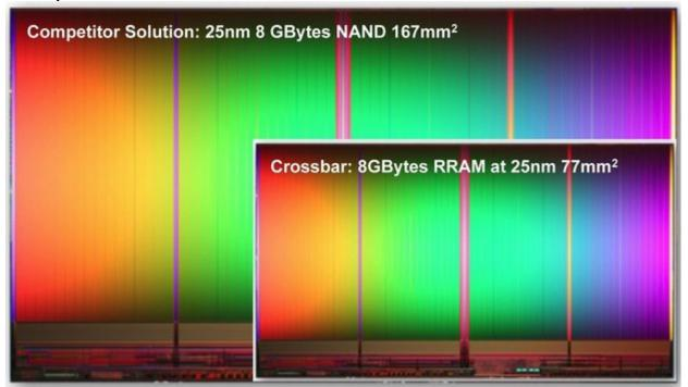
RRAM will be able to use silicon wafers that are half the size used by current NAND flash fabricators. In a single chip, it has nearly 10 times the capacity of NAND flash and uses 20 times less power to store a bit of data."
