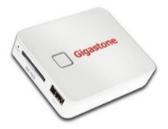
The Gigastone Smartbox (http://www.gigastone.com/; \$45) combines an SD memory socket with an 802.11 b/g/n hot spot and a lithium ion battery. It allows up to six Wi-Fi devices to connect and share up to 32 GB of SDHC memory, providing handy file sharing and streaming. It can even provide a back-up power source for USB-powered devices.
