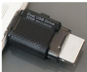
In this context, a dual USB drive is a device that has two USB connectors. In the case of the SanDisk Ultra, as shown in the picture, it has a standard USB type A male and a standard micro USB male connector. The connections are not to be used at the same time.
